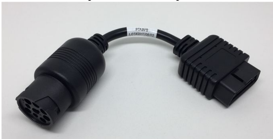
9pin to OBD-II adapter
